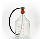
DI-111-A Water Trap for Liquid Digestion and Scrubber
