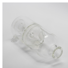
KD-030-A1 Glass Splash- head for Standard Analysis
